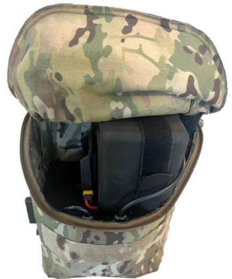
Receiver fully integrated within Power Unit
